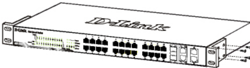
Figure 2 – Attach the mounting brackets to the Switch
