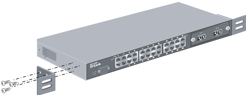
Figure 2- 2A. Attaching the mounting brackets to the switch
