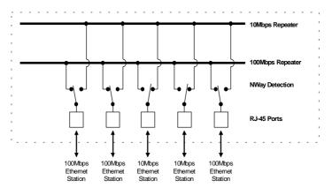
If there is a DFE-908x hub present in the stack, its built-in switch serves as a bridge between the two independent segments.
