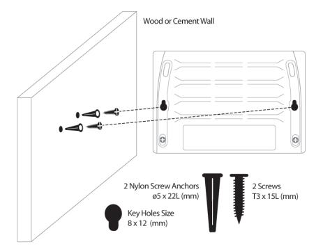
(1) 3/4 inch minimum for wood wall(2) 3 inch minimum for cement wall.
