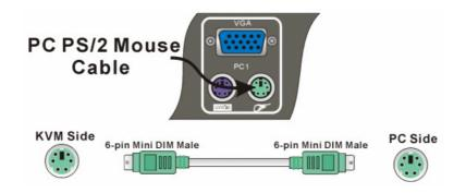
Step 6. To finish the hardware installation, connect the PS/2 keyboard cables from your computers to the DKVM-2/4 unit. Connect a keyboard cable (6-pin Mini DIN Male / Male) to the PC and to the connector with the keyboard symbol on the rear panel of the DKVM-2/4 unit. Repeat this for all PCs.
