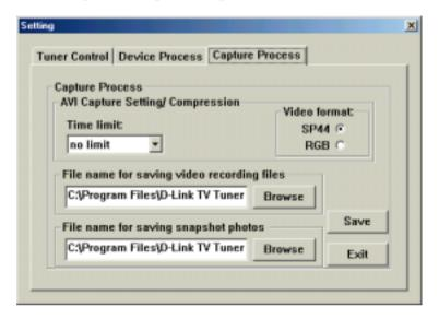
The "Time limit" drop down box allows you to select the recording time limit from 30 seconds up to 120 minutes or no limit. All files are saved in AVI format. You can also change the **Video Format** to SP44 or RGB.
