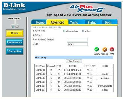
An Infrastructure network includes a router or an access point; an Ad-Hoc network is a Peer-to-Peer network with a direct communication between two DWL-G820s.
