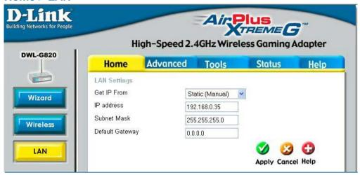
LAN is short for Local Area Network. This is considered your internal network. These are the IP settings of the LAN interface for the DWL-G820. These settings may be referred to as private settings. You may change the LAN IP address if needed. The LAN IP address is private to your internal network and cannot be seen on the Internet.
