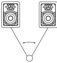
For best stereo imaging, we recommend that the units be placed so that the tweeters are as close as possible to the ear level of a seated listener. As this is not always possible in keeping with aesthetic design of a particular room, MODEL W625 and W825 In-Wall Loudspeakers were designed with a pivoting tweeter which rotates to allow you to "aim" the high frequencies toward the listening position.
