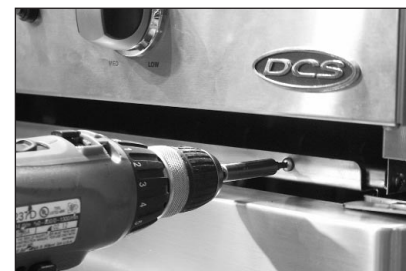
Secure grill to the front of the cart with Phillips-head screws (provided).
