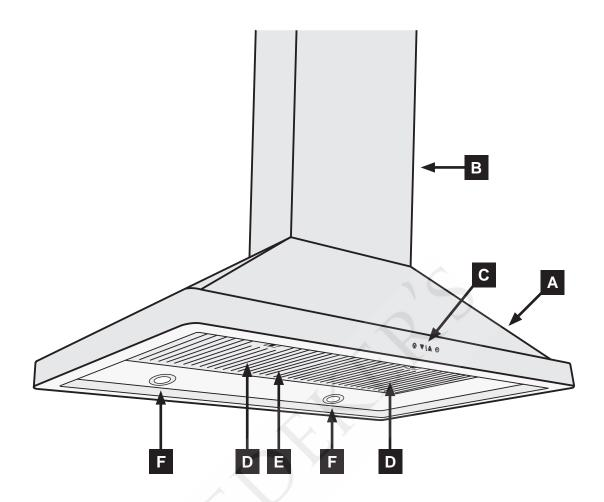
A HOOD - The hood directs heat and smoke into the blower system located inside the unit. The blower system forces heat and smoke into the duct inside the chimney **B** which vents to the outside. The filter, the lights and main power switch are located on the bottom of the hood. The blower system on some models, consists of more than one blower. See the table below.
