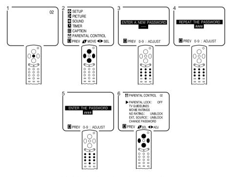
You can set each individual settings using  $\triangle CH \vee$  and  $\triangleleft VOL \triangleright$  buttons.
