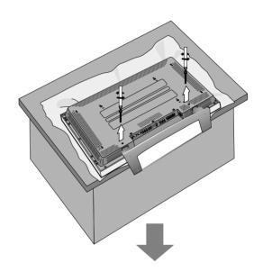
• Pull the stand away from the plasma display to disassemble.
