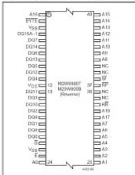
Figure 2B. TSOP Reverse Pin Connections
