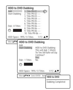
When dubbing process is completed, the tray will be open automatically.
