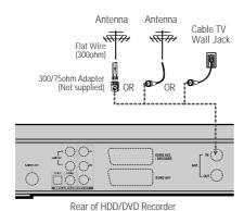
If your cable wire is connected to your TV without a converter or descrambler box, unscrew the wire from your TV and attach it to the RF IN (FROM ANT.) jack on the rear panel of the HDD/DVD Recorder. Use the supplied RF cable to connect between the HDD/DVD Recorder's OUT (TO TV) jack and the antenna input jack on your TV. With this connection, you can receive all midband, superband, and hyperband channels (all cable channels).
