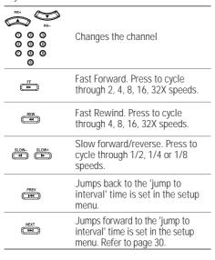
If you are using the default value of "Setup -> Preferences -> Hard Disk -> Buffer mode -> Refresh", and change Channels, the Time shifting buffer data will be lost. No message will be provided prior to doing so. However, if you set "Setup -> Preferences -> Hard Disk -> Buffer mode --> Preserve", and change Channels, the Time shifting buffer data will be maintained.
