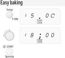
Set one of the 12 temperature levels. Press the button 1 - 12 times.
