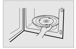
7 The roller guide and oven cavity floor should be cleaned regularly to avoid excessive noise. Simply wipe the bottom surface of the oven with mild detergent water or window cleaner and dry. The roller guide may be washed in mild sudsy water.
