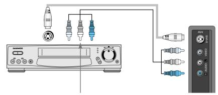
Connection is not necessary in Mono mode.
