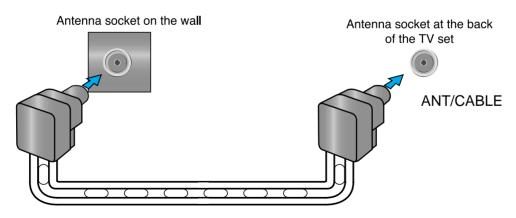
Feeder cable connection with the combining adapter
