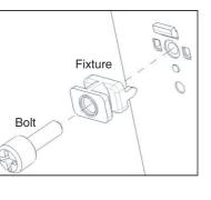
2. Align door handle with fixture and pull the handle down.
