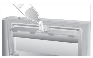
1. Open the cover cap and pour water into the water tank.
