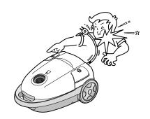
Make sure a dust bag and a motor protection filter are always inserted.
