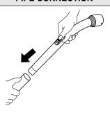
To connect the nozzle, hold the tubes and the handle: insert the narrowed section into the wide section.
