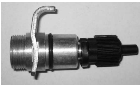
Gear installed on new Ford adaptor
