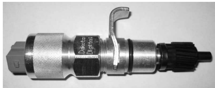
New sensor installed on adaptor
