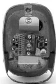
LED assembly mounted in an original housing.
