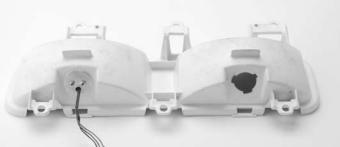
8. Install the lens and/or re-assemble the tail light housing, insuring all gaskets are intact and in place. Install the tail light housing back into the vehicle. You are now ready to wire the LED assembly into the vehicle tail light harness.
