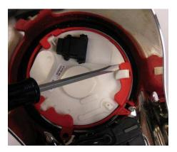
Insure that the rubber gasket is still in the dash or remove from factory gauge and place back on dash
