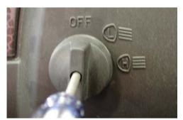
2. Remove the Phillips screw holding the original head light switch cover in place.
