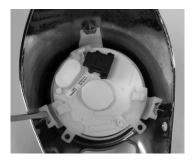
Remove the rubber gasket from the factory gauge bezel
