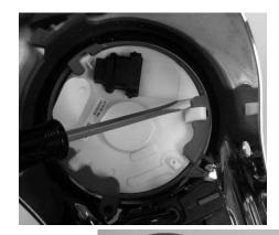
Insure that the rubber gasket is still in the dash or remove from factory gauge and place back on
