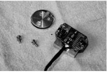
6. Pass the wires through the housing where the original bulb and socket where.
