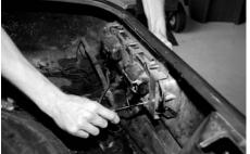
3. Next remove the lens to gain access to the housing. There are six screws that hold the housing halves together, remove the screws and separate the halves carefully.
