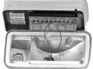
10. Fasten the lens back on with the four original screws.
