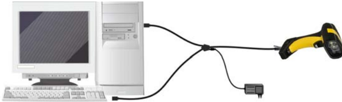
Figure 5 – PC Wedge Connection
