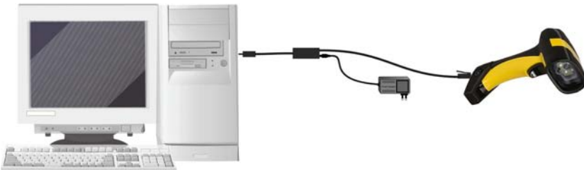
Figure 7 – PC USB connection
