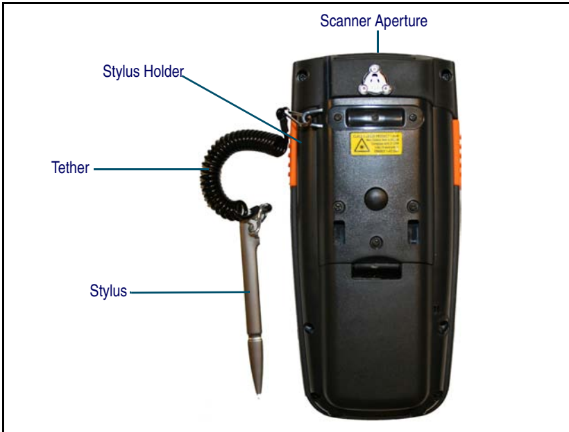
Figure 7. Back View of a Pegaso with a Stylus
