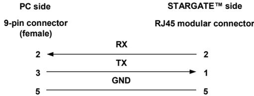
**Figure 7 - RS232 Pinout**
