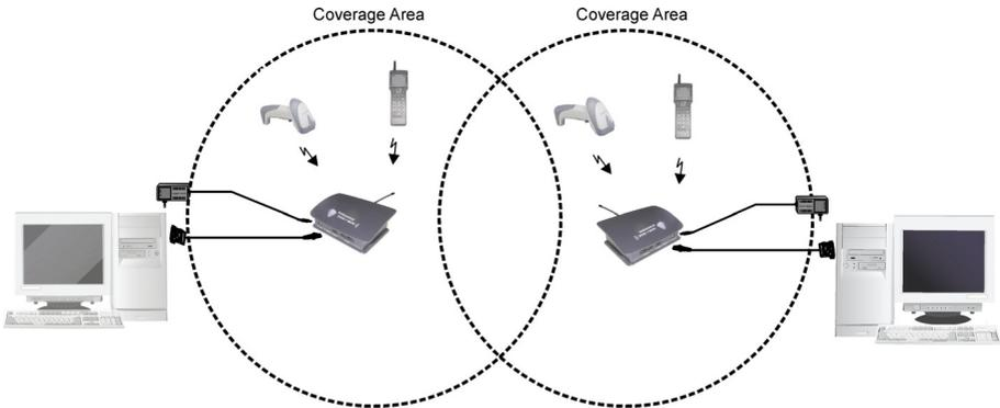
**Figure 15 - Separate STAR-System(s)™ with Overlapping Coverage Areas**
