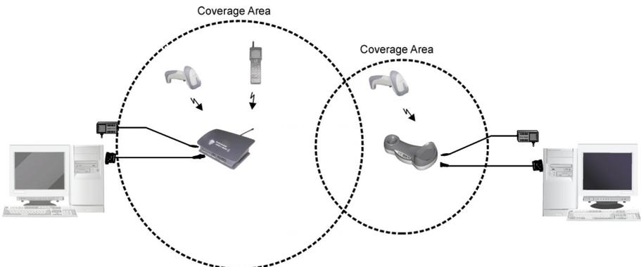
**Figure 16 - STAR-System™ and Other RF Networks Having Overlapping Coverage Areas**
