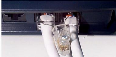
Figure 12 - Linking the Cable Shields
