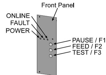
**Note:** More information on the Front Panel can be found in Section 3.4 of the Operator's Manual.
