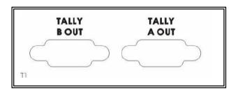
Connect to Datavideo TLM-404 4"x4 TFT LCD or connecting an certain adaptor cable to control the Tally interface of video input source devices, such as Came
