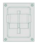
T-bar is for performing effect transitions manually. It can be either all the way up, all the way down, or anywhere in between. To enable SE-800 T-Bar, the T-Bar on RMC-90 need to be set at either end of its travel.
