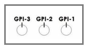
GPI Trigger outputs to control DV Bank
