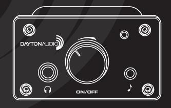
**Thank you** for purchasing the Dayton Audio DTA-120 Class T Digital Audio Power Amplifier. This amplifier features the Tripath TK2050 chipset that provides 60W continuous power per channel (120W total) into an 4 ohm load. Class T amplifiers using Tripath's proprietary Digital Power Processing ™ technology offer the audio fidelity of a Class AB amplifier while providing the power efficiency of a Class D.
