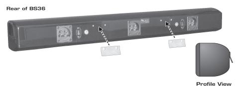
Step 2: Identify mounting location and attach wall bracket to the wall using supplied drywall screws. Do not use nails. Attach one end first then pivot until bubble is level. Mark holes and install remaining screws. When using the supplied "Wall Dog" screws it is not necessary to locate a wall stud.
