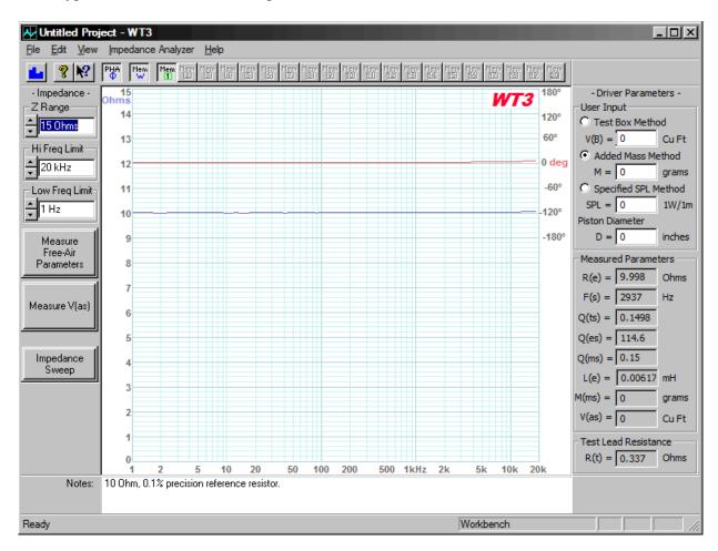
An ideal resistor would have a perfectly flat impedance response at exactly the rated value of the resistor. Notice that the measured impedance (shown above in blue) of this 10 Ohm precision resistor is almost perfectly flat over the audio frequency range. This is not unusual for a resistor because real resistors typically do behave largely as ideal resistors. The impedance phase response is essentially flat
