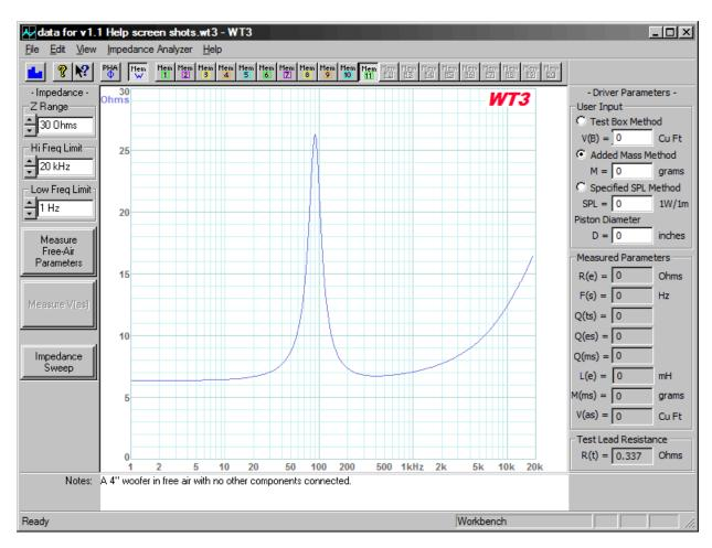
With a DC resistance of 5.5 Ohms this would most likely be considered to be an 8 Ohm driver. So let's set the resistor value to about 8 Ohms. Looking in my parts bin I see the closest values on hand are 5 and 10 Ohms. Let's use 10 Ohms so that we tend to under compensate. We'll select the capacitor value by starting too low and stepping up the capacitor until the impedance response looks about as flat as
