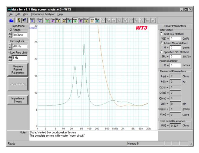
Finally, here is a screen shot showing the same system with the woofer in a short circuit fault condition (lower blue trace). As we see in these examples often a system fault is most easily detected by comparing the suspect system to a known good system.
