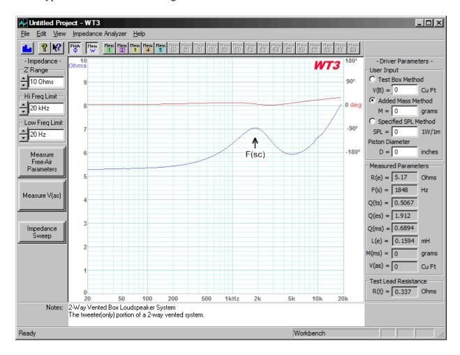
We can read the tweeter's resonance frequency, F(s) (or, more strictly F(sc)), directly from the impedance plot or note the value at the Measured Parameters F(s) field. Just as with a closed box, the system's Q(tc) is read from the Q(ts) field. Similarly for the electrical and mechanical Q's. The above tweeter is seen to have a resonance of 1.848 kHz and Q(tc) of .5067.
