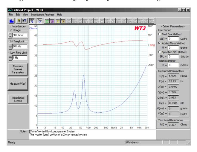
In order to read the vent tuning frequency, F(b), more precisely we can adjust the frequency display limits to zoom in on the frequency range containing the two impedance peaks as shown below:
