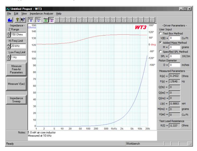
An ideal inductor would have an impedance of zero Ohms at the lowest frequencies and then the impedance would rise with increasing frequency. The phase response of the inductance depends on the exact circuit in which the inductor finds itself. At very low frequencies (1 Hz) the impedance measurement reveals the DC resistance of the inductor. Notice that the impedance (blue) of the real inductor measured above is near zero at low frequencies and rises at high frequencies as expected. The
