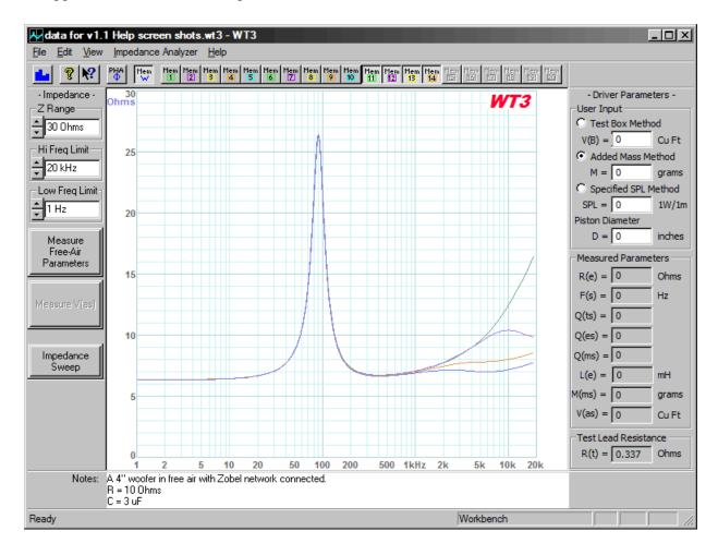
Below we see the effect of increasing the capacitor to 5 uF in the lowest (blue) trace. It seems we have gone too far with the increase to 5 uF. The impedance in the 2 to 3 kHz range has been reduced to the DC resistance value and is now rising above the previous measurement with the 3 uF capacitor. This rise may be due to an interaction with the voice coil inductance. It looks like the 3 uF capacitor will be the best overall choice to tame the driver's high frequency impedance.
