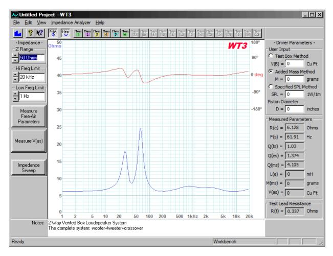
We can see that this system employs a vented woofer system with the vented enclosure tuned to about 40 Hz. Even with a minimum impedance of just over 6 Ohms this would often be considered to be a nominal 8 Ohm loudspeaker system.
