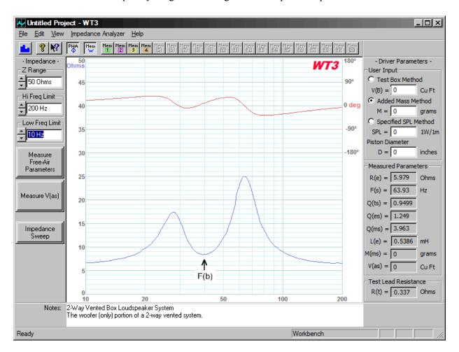
At this screen we can determine that F(b), the tuning frequency of the vented box, is approximately 40 Hz by locating the impedance minimum between the two peaks and reading the frequency where the minimum occurs. The closely zoomed view makes it easier to read the frequency from the scale below.
