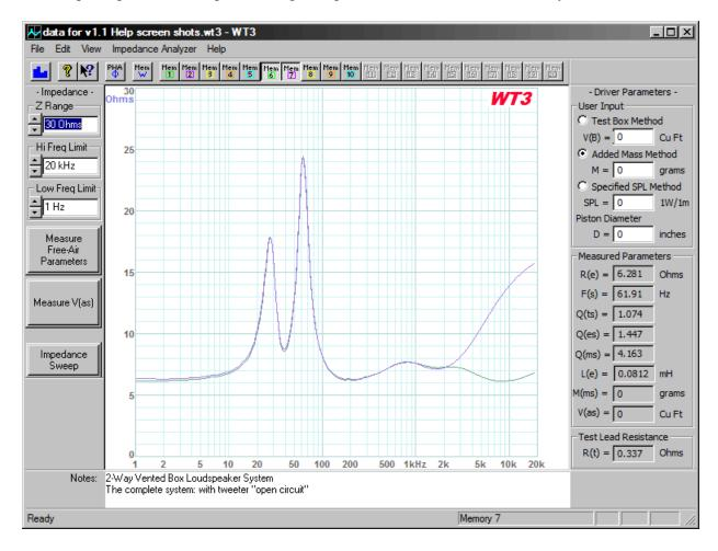
In the screen below you see the same system as above but this time with a shorted tweeter. The green (upper) plot again shows the normal impedance response of this system. The yellow (lower) plot shows the system with a shorted tweeter. The system with the shorted tweeter appears to have a suspiciously low impedance above 4 kHz or so but when compared to the normal response (green) it is easy to see there is a problem.
