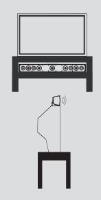
If placed on a shelf under a TV, adjust the leveling feet (screwed all the way in) to aim the speaker up towards the listeners.
