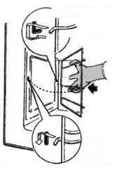
To remove the side racks, lift and pull out the front, slide the rack forwards and lift free. Fit in reverse order
