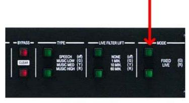
**2.** Hold this **MODE** button until the filter LEDs flash all the way across.
