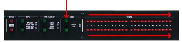
**7.** Press the **BYPASS** buttons so that they are both lit red (bypassed).
