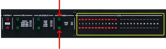
Press the **LIVE FILTER LIFT** buttons to increase the # of "Fixed" filters for each channel. Press the **TYPE** buttons to decrease the # of "Fixed" filters for each channel. The default of 12 Fixed and 12 Live is a good place to start.
