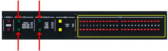
**5.** Press the Mode buttons. They should now be lit green. The filter LEDS will indicate how many of these total filters will be allocated as "Fixed" filters.
