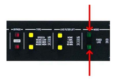
**14.** Disengage the Bypass buttons (LEDs off).
