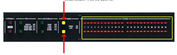
**4.** Select how many total filters that you want active. The default of 24 is a good place to start. However, if you want to change the total # of filters, press the **LIVE FILTER LIFT** button to increase the # of total filters for each channel or the **TYPE** button to decrease the total # of filters for each channel.
