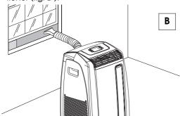
Thanks to the locking pins, it's possible to use the window bracket also for sliding windows. Position the hole of the bracket so to allow a correct installation of the exhaust hose (see figure **C**).
