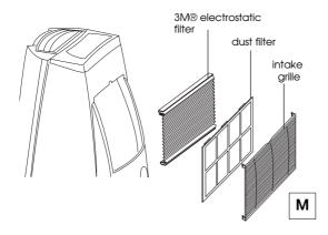
Use a vacuum cleaner to remove the dust collected on the filter.
