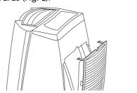
2. Remove the dust filter by detaching it from the grille (Fig. **M**). Remove 3M® electrostatic filter if it is mounted.
