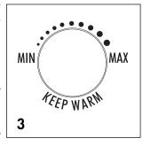
temperature by turning the knob to the desired position (fig. 3). Some models have a FRESHNESS indicator that shows how long it has been since the last coffee was brewed. When the coffee is just made, the light turns green, and every 20 minutes a triangle segment of the light becomes red.
