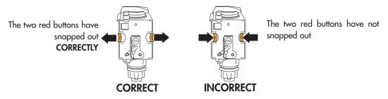
**NOTE 1:** If the infuser is not inserted correctly until it clicks into place and the two red buttons have not snapped out, the service door cannot be closed.
