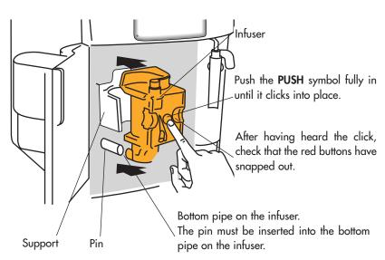
Check that the two red buttons have snapped out, otherwise the door cannot be closed.
