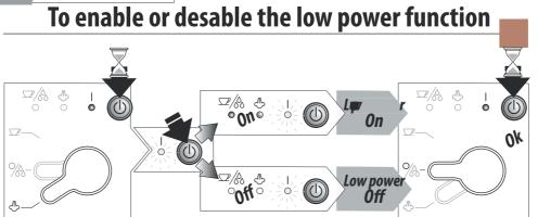
When LOW power is enabled, the device will automatically activate LOW POWER after 15 minutes and subsequently go into standby mode.
