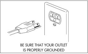
This appliance must be grounded. In the event of an electrical short circuit, grounding reduces the risk of electric shock by providing an escape wire for the electric current
