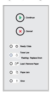
**NOTE:** If the light is blinking, see "The Toner Low/Replace Drum light is blinking." on page 51.
