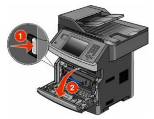
2 Press the button on the base of the photoconductor kit. Pull the toner cartridge up and out using the handle.
