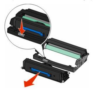
**4** Unpack the new photoconductor kit. Be careful not to touch the photoconductor drum.
