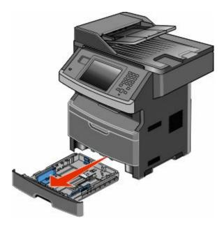
**2** Squeeze and slide the guides to the correct position for the paper size you are loading.
