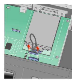
**b** Remove the screws holding the printer hard disk in place.
