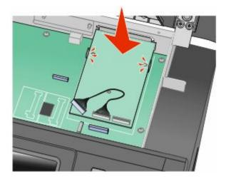
**6** Install the ISP onto the plastic tee. Angle the ISP over the plastic tee, and then approach the plastic tee so that any overhanging connectors will pass through the ISP opening in the system board cage.
