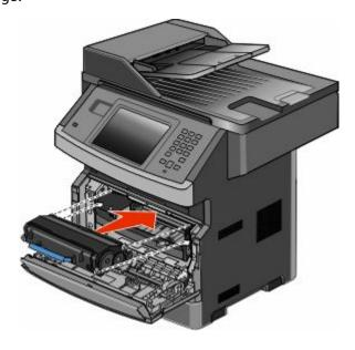
**7** After you replace the photoconductor kit, reset the photoconductor counter. To reset the counter, see the instruction sheet that came with the new photoconductor kit.
