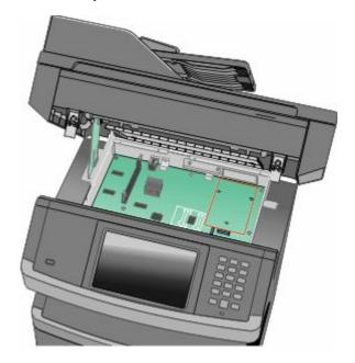
**Note:** If an optional printer hard disk is currently installed, then the printer hard disk must first be removed. To remove the hard disk:
