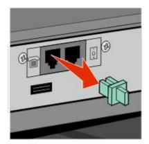
4 Connect your telecommunications equipment directly to the printer EXT port **1**.
