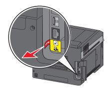
**8** Temporarily connect a USB cable between the computer on the wireless network and the printer.
