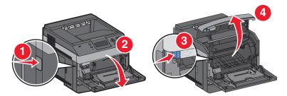
**3** Lift and pull the toner cartridge out of the printer.
