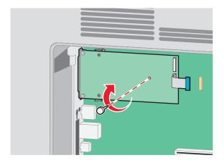
**9** Attach the two provided screws to secure the ISP mounting bracket to the system board cage.
