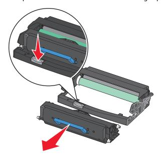
**4** Unpack the new photoconductor kit. Be careful not to touch the photoconductor drum.
