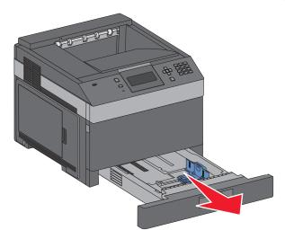
**2** Squeeze the width guide tab inward as shown, and move the width guide to the correct position for the paper size being loaded.
