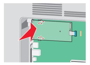
**8** Insert the long thumbscrew and turn it clockwise enough to hold the ISP in place, but do not tighten the thumbscrew at this time.
