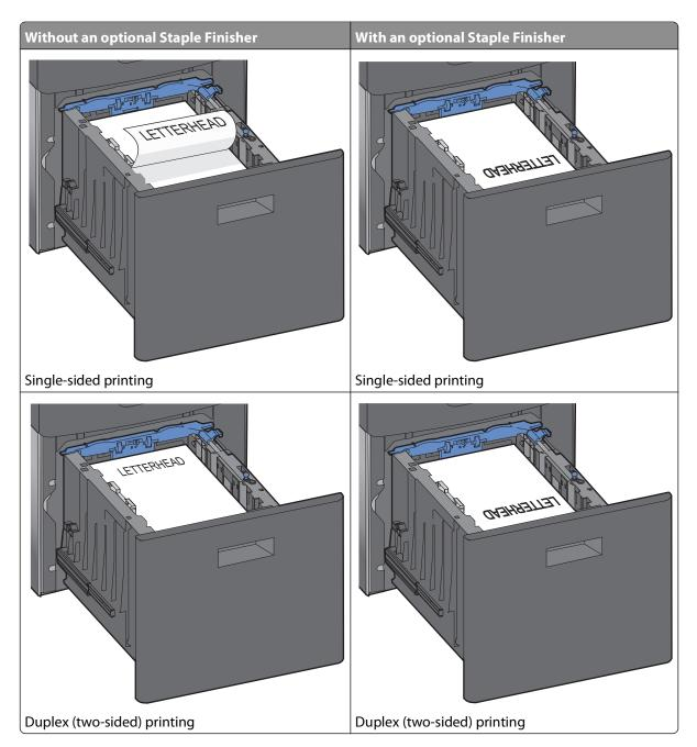
**Note:** Notice the maximum fill line on the side of the tray which indicates the maximum height for loading paper. Do not overload the tray.
