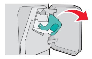
**3** Use the metal tab to lift the staple guard, and then remove any loose staples.
