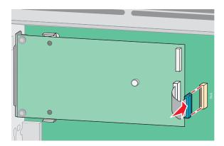
**12** If a printer hard disk was previously installed, then attach the printer hard disk to the ISP. For more information, see "Installing a printer hard disk" on page 31.
