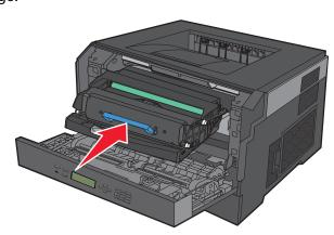
**7** After you replace the photoconductor kit, reset the photoconductor counter. To reset the counter, see the instruction sheet that came with the new photoconductor kit.
