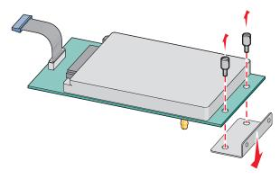
**b** Align the standoffs of the printer hard disk with the holes in the ISP, and then press downward on the printer hard disk until the standoffs have seated into place.
