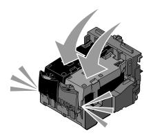
**9** Lift the printer unit, and hold the scanner support up while lowering the printer unit until it is completely closed.
