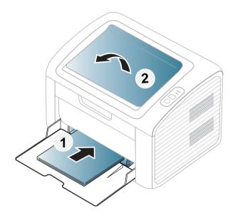
Squeeze the paper width guide and slide it to the edge of the paper stack without causing it to bend.
